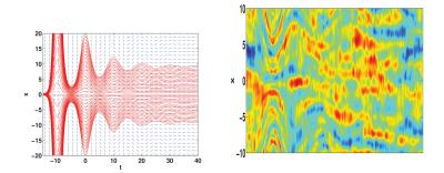
Trajectories and directional field of a simple dynamical flow representing damped oscillations *(Left)*. Dynamic spatio-temporal random fields X(x, t) for  $\lambda = 0.5$  and  $\sigma^2 = 0.5$  *(Right)*.
