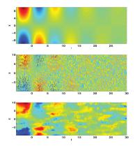
Velocities of dynamical flow (*Top*) vs. velocities of stochastic field: unfiltered (*Middle*) estimated by the median filter (*Bottom*).  $\lambda = 0.5$  and  $\sigma^2 = 0.5$ .
