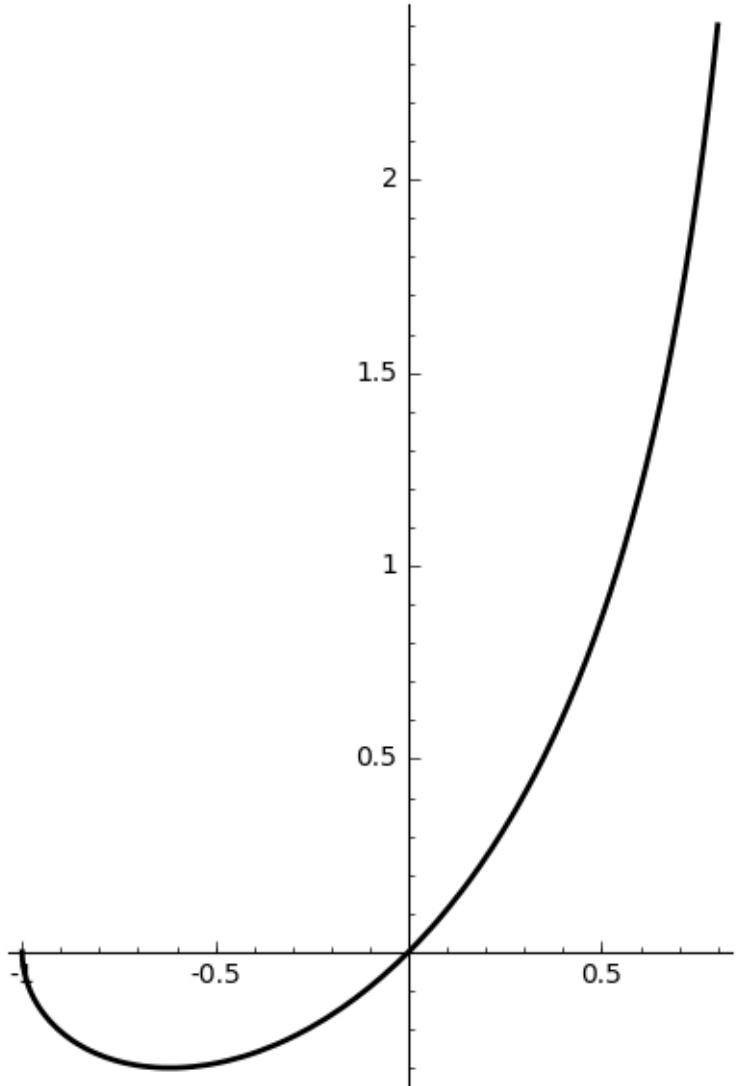
In [7]: `parametric_plot(((x^2-1)/(x^2+1),(x^3-x)/(x^2+1)),(x,-3,3),color='black',thickness=2)`
