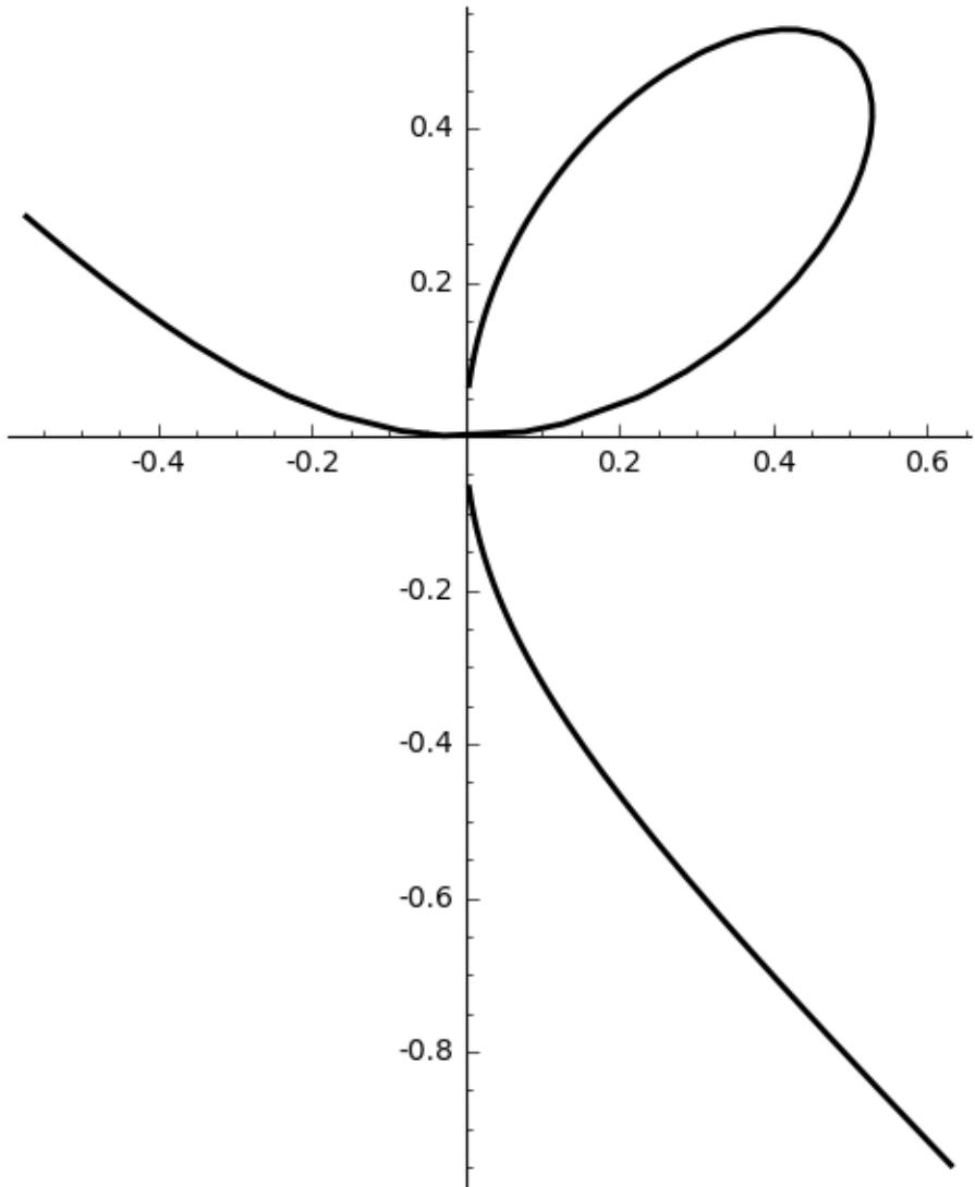
In [13]: `parametric_plot((x*ln(x),ln(x)/x),(x,0.2,5),color='black',thickness=2)`
