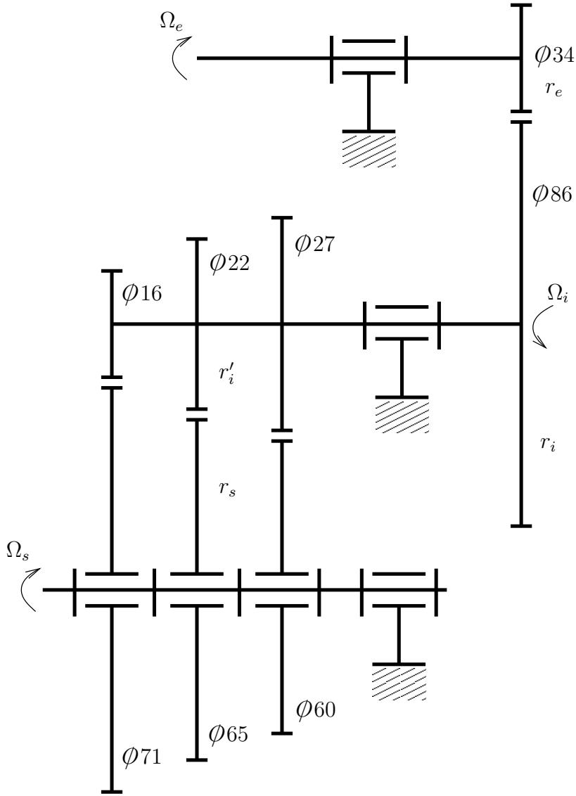
$$\Omega_e r_e = \Omega_i r_i \quad \text{et} \quad \Omega_i r'_i = \Omega_s r_s$$
