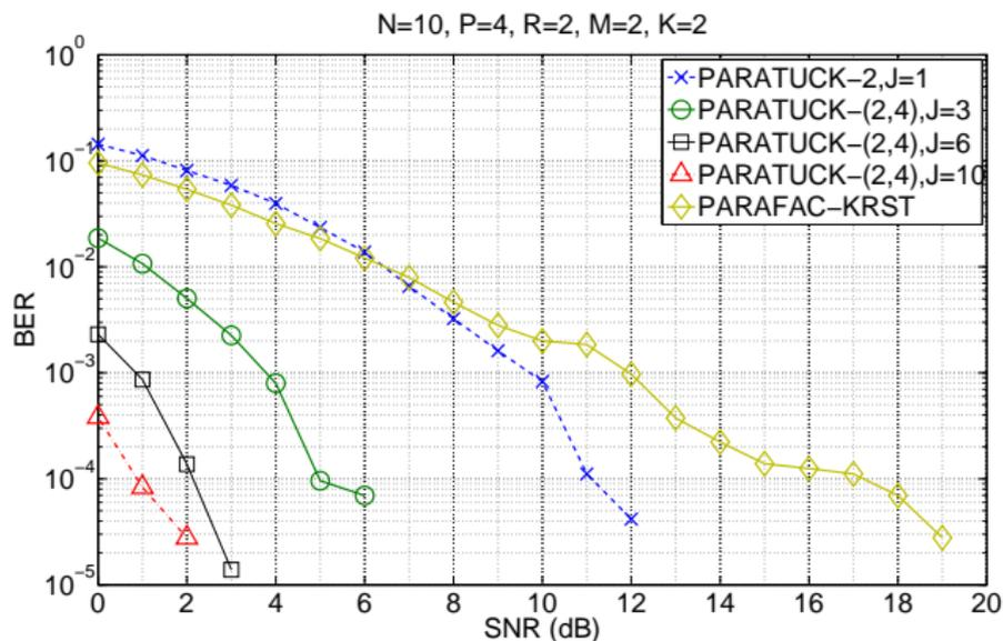
Figure : Influence of the spreading length: BER versus SNR.
