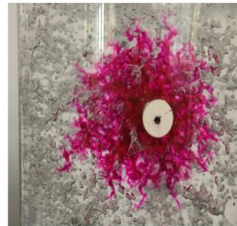
Dye plume propagation in a irregularly shaped grains of PAM
