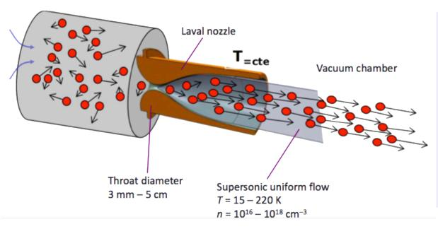
Laval nozzle controls expansion of carrier gas: avoids problems of other cooling methods:
