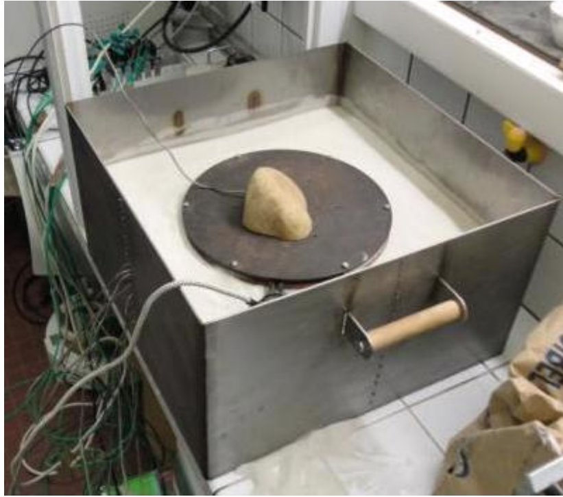
Figure 5.1: Experimental hearth. The sand is fully saturated with water.
