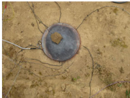
Figure 11. Electrical plate is put on the soil.
