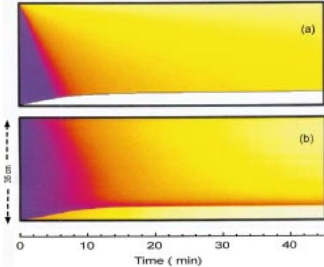
**Fig. 3.** Space-time plots of (a) predicted liquid content, equation (4), assuming Plateau border-dominated dissipation and neglecting capillarity, and (b) diffuse transmission of white light through an actual foam.
