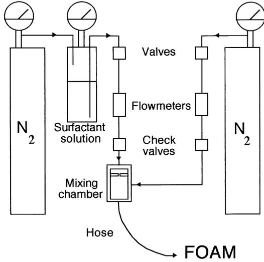
**Fig. 1.** Apparatus for the production of foam. Surfactant solution is forced through a small hole in the mixing chamber, where the resulting jet mixes turbulently with a continuous supply of gas. By controlling the liquid:gas flow rates, the liquid content of the foam may be chosen as desired.
