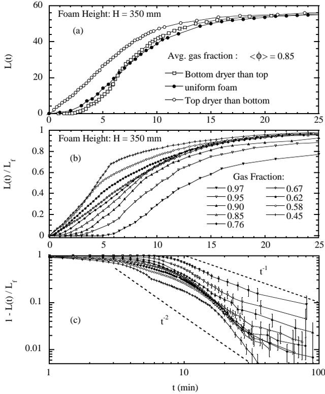
**Fig. 2.** Height of drained liquid underneath a foam *vs.* time after production for (a) nonuniform initial liquid content and (b,c) uniform but variable initial liquid content. The latter are normalized by the final liquid height,  $L_f = L(\infty)$ .
