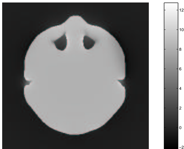
Figure 16: Induced magnetic field in \mu T on an axial slice of the brain crossing the nasal fossa.
