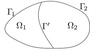
$$u \in W^{1,p}(\Omega) \Leftrightarrow \begin{cases} u_1 \in W^{1,p}(\Omega_1), u_2 \in W^{1,p}(\Omega_2), \\ \text{et } \gamma_0 u_1|_{\Gamma'} = \gamma_0 u_2|_{\Gamma'}. \end{cases}$$
